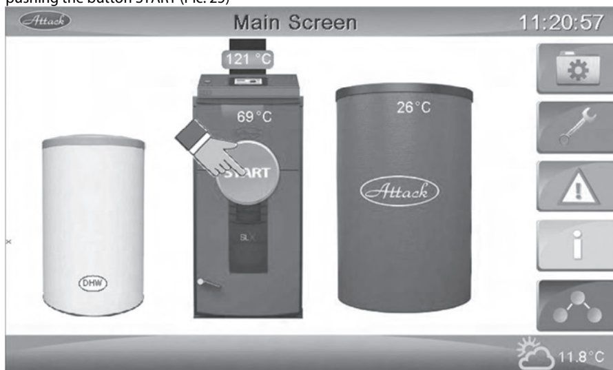
Pic. 25 Boiler start on
