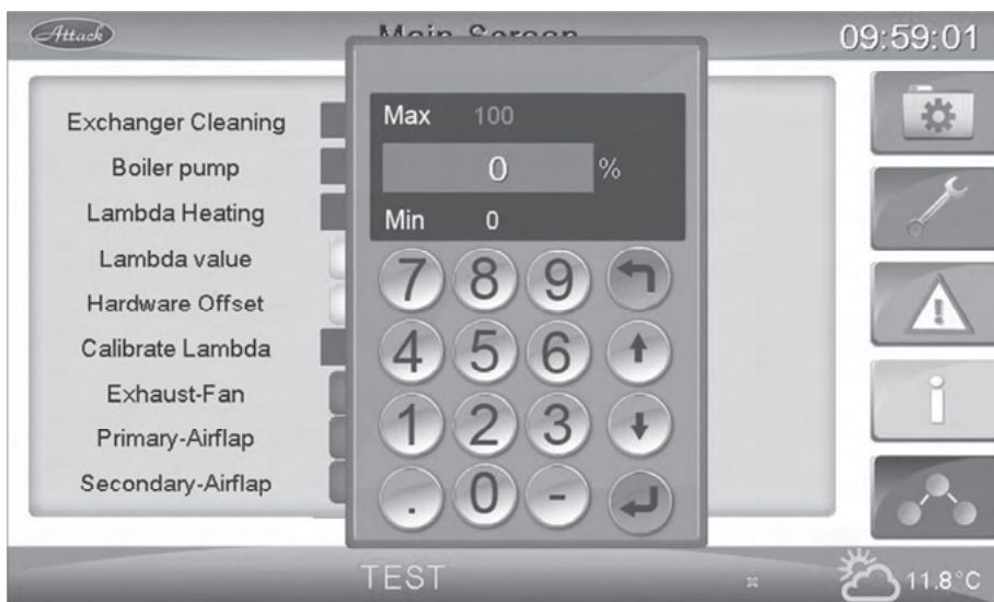
Pic. 23 Testing activation of devices unable to be changed (modulated)
