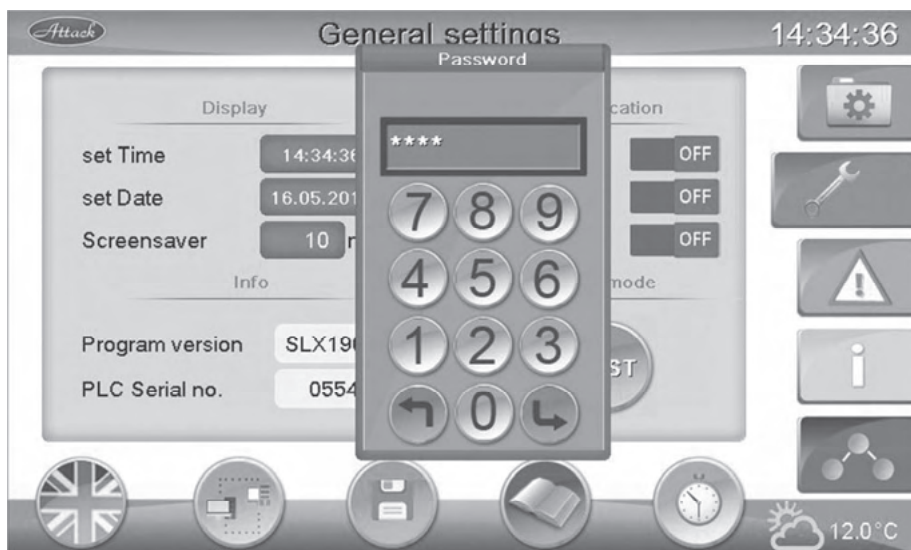
Pic. 53 Access to advanced parameters
