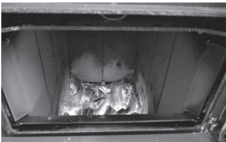
Pic. 13 Height of the live coals suitable for stoking.
