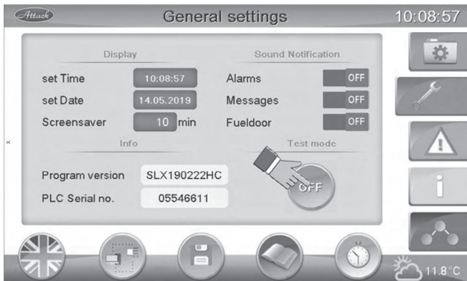
Pic. 24 Finishing of the boiler's test mode
