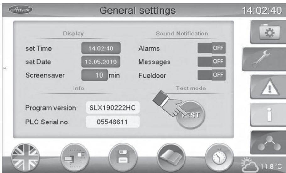
Pic. 20 Entry into TESTMODE
