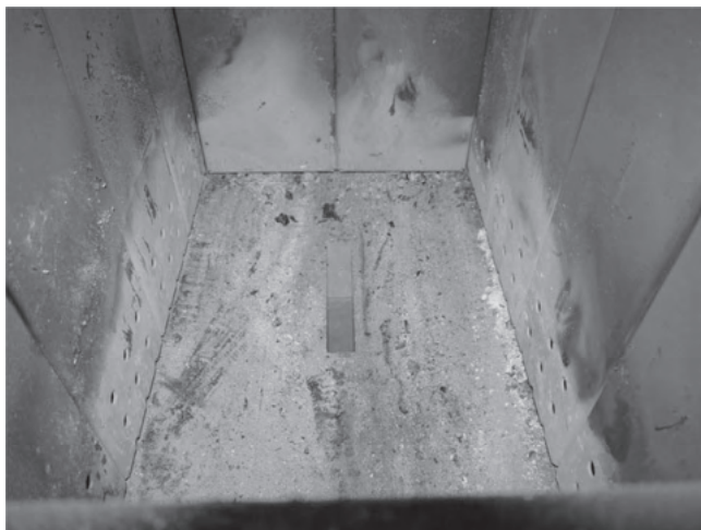
Pic. 6 Correctly cleaned feeding chamber
