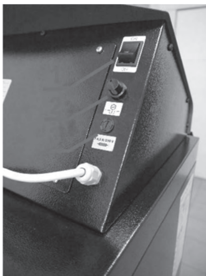
Pic. 17 1 – main switch, 2 – emergency thermostat, 3 – fuse (F6,3 A)
